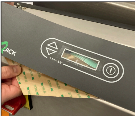
22. Pull the cover out from underneath the foil. Do not lift the foil to much, it can break the foil. Check the display connector is placed through the hole.
