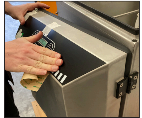
21. Press the foil evenly on to the service door.
