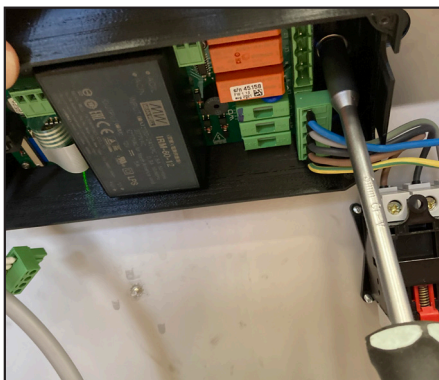
32. Adjust the black box placement by loosening the two nuts located on each side of the black box and move the box into place.
