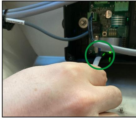
11. Place and hold the upgrade tool connector correctly on the control unit connector.
