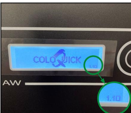
7. The current software version number is visible on the lower right corner of the display when turned on.
