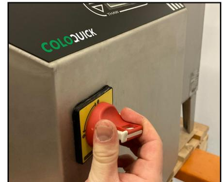
6. Turn on the machine. Make sure there is water in the water bath to prevent the heating element from overheating.
