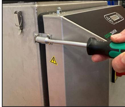
2. Remove the nuts to unlock the service door. **DANGER! When the service door is open there is a risk of electric shock!**
