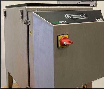
1. Place the THAW unit in an optimal height for easy access. Open top lid to deactivate the lid switch. **Make sure there is water in the water bath!**
