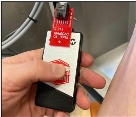
13. Press and hold the button on the upgrade tool for a few seconds.
