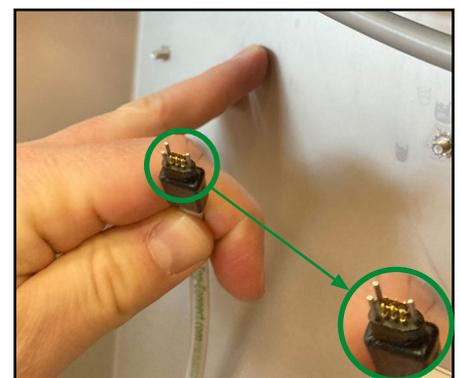
9. Make sure the upgrade tool connector is positioned exactly as shown on this picture with two pins to the left side.
