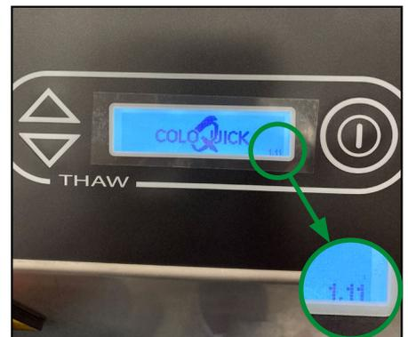
18. Turn the THAW unit off and on to check if the version number is correct.
