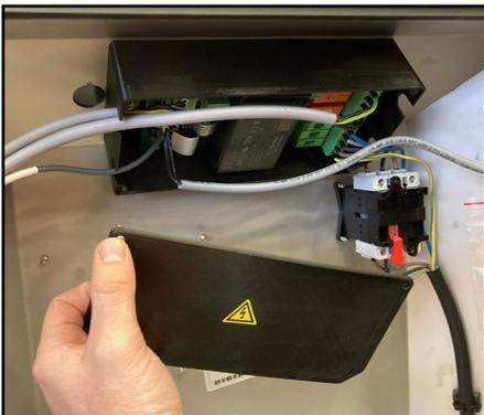
4. Remove the four screws and remove the lid from the black box. **DANGER! Risk of electric shock!**
