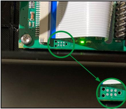
10. The control unit connector is placed close to the lower left corner. As marked with the circle above.
