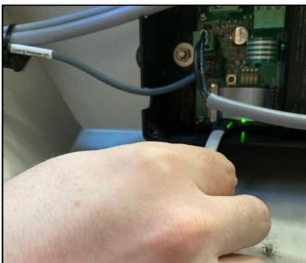
16. Remove the upgrade tool connector.
