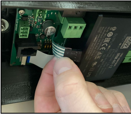
10. Unplug the display connector from the control unit.
