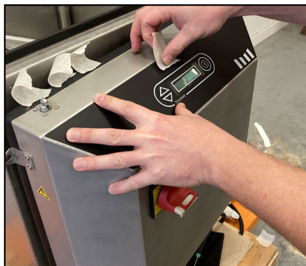
17. Hold the display in place and attach it to the service door with the prepared tape pieces.
