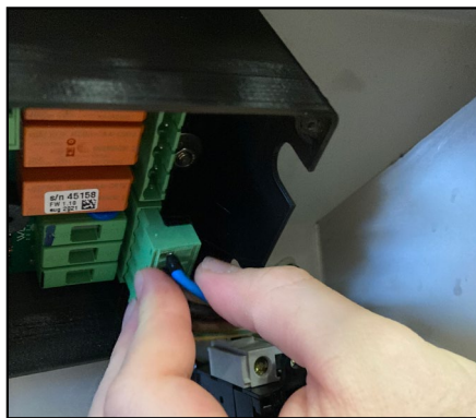
29. Plug in the green plug placed in the lower right corner.
