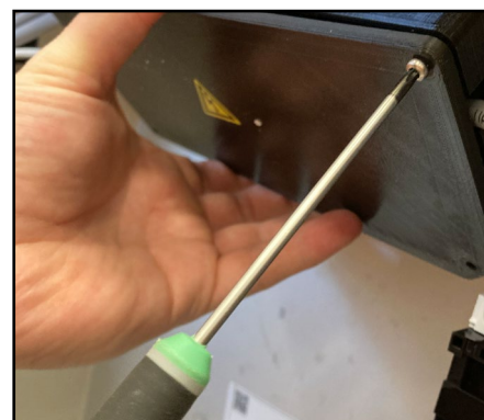
36. Close the black box with the lid and four screws.
