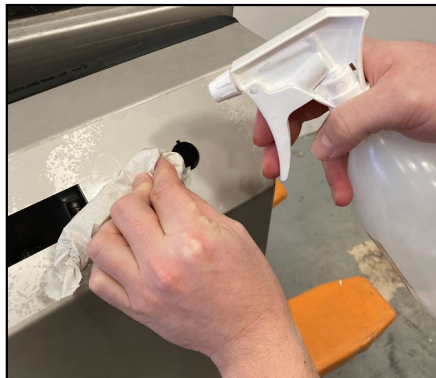
14. Clean and remove the remaining glue of the service door by using paper towel and isopropyl alcohol.
